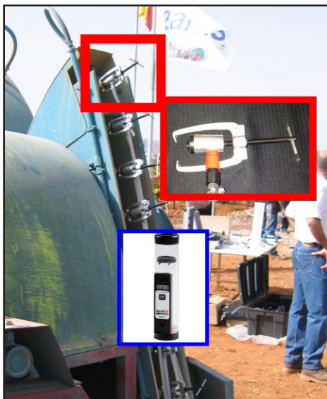
Figure 3 - Using the proper nozzle clamps (top) and flow meter (bottom) make this step easier and faster.
