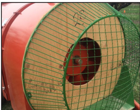
Figure 2 – Plywood ‘donut’ applied to the rear of a sprayer to restrict air intake. Photo by Jaime Ramon, WSDA
