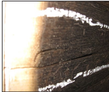
Figure 4 – Cracking at the edge of the croze. Photo by Tom Collins.
