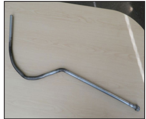
Figure 6 - Shop-built "persuader" for reinserting barrel heads. Photo by Tom Collins.
