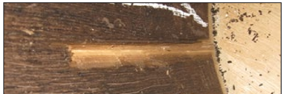
Figure 5 – Chipping of a stave that occurred during routing of the croze. Photo by Tom Collins.
