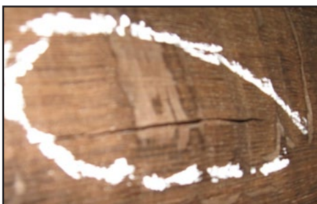
Figure 3 – Blistering in a barrel stave. Photo by Tom Collins.
