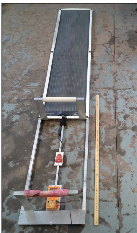
Figure 1 – The Paso panel was constructed with a 6' solar panel, multi-meter, and temporary switch. A bubble level was used to maintain orientation during data collection.
