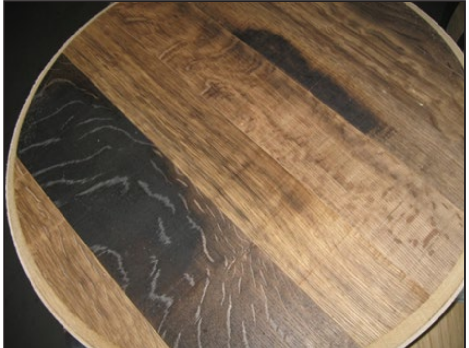
Figure 1 – Inconsistent milling and toasting in a barrel head. Photo by Tom Collins.
