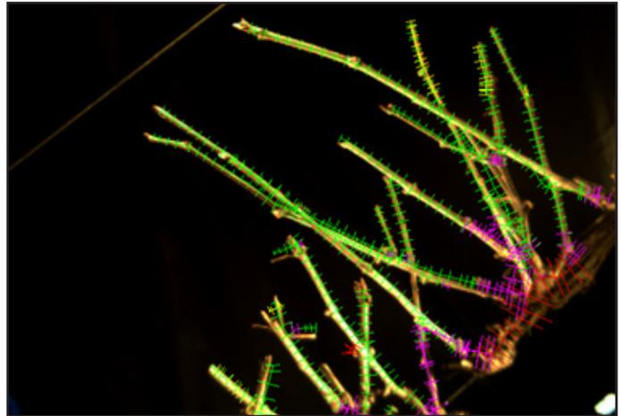
Figure 2- 3D model of the vine projected onto a 2D front camera image.
